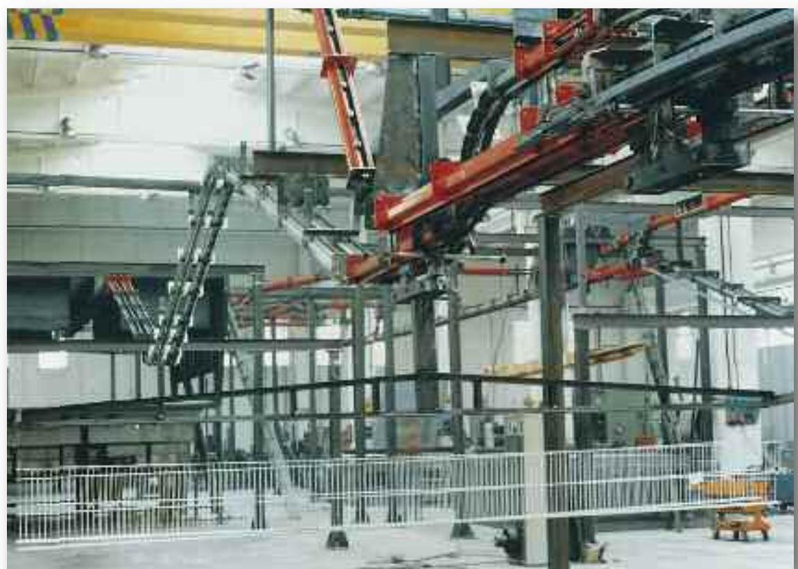
*Detail of the conveying system of a fluidized bed plant for the coating of 3600 mm wide pieces and the production of about 3600 Kg/h installed in the U.S.A.*
