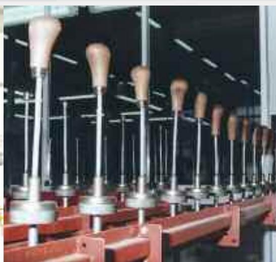
Painting plant for application of wet paint for automobile gear shift lever knobs
