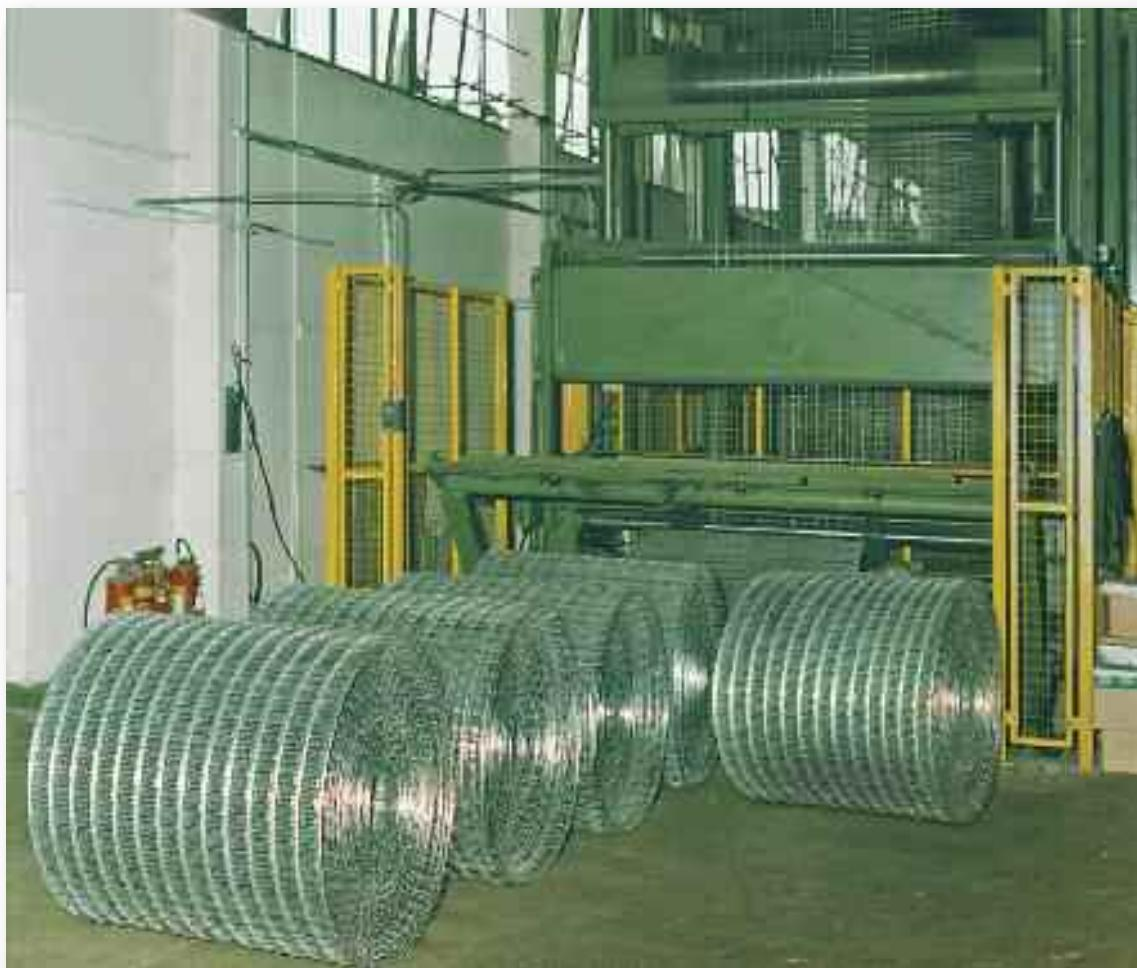
*Auxiliary reel-off and winding devices for wire mesh*
