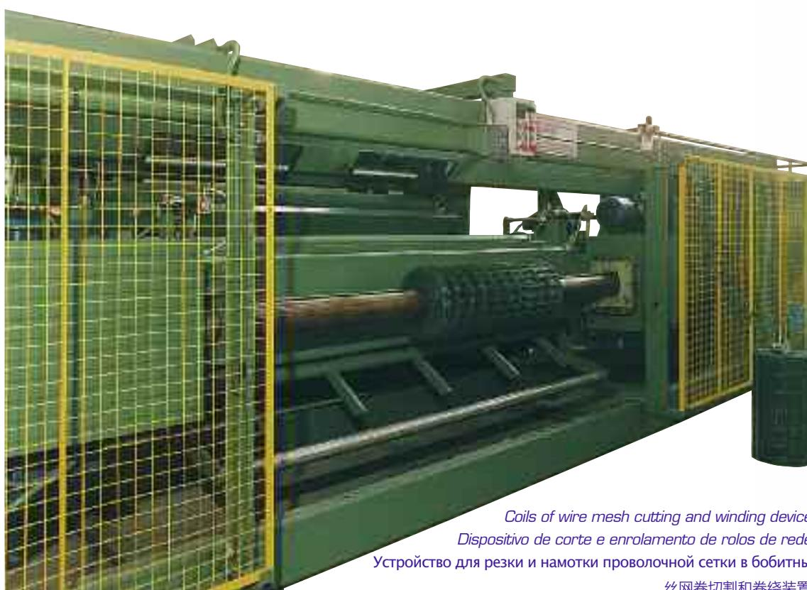
*Coils of wire mesh cutting and winding device*
