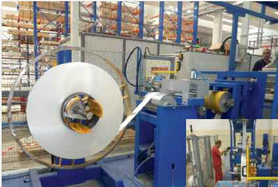
*Coil coating plant with fluxing application on aluminium belts*
