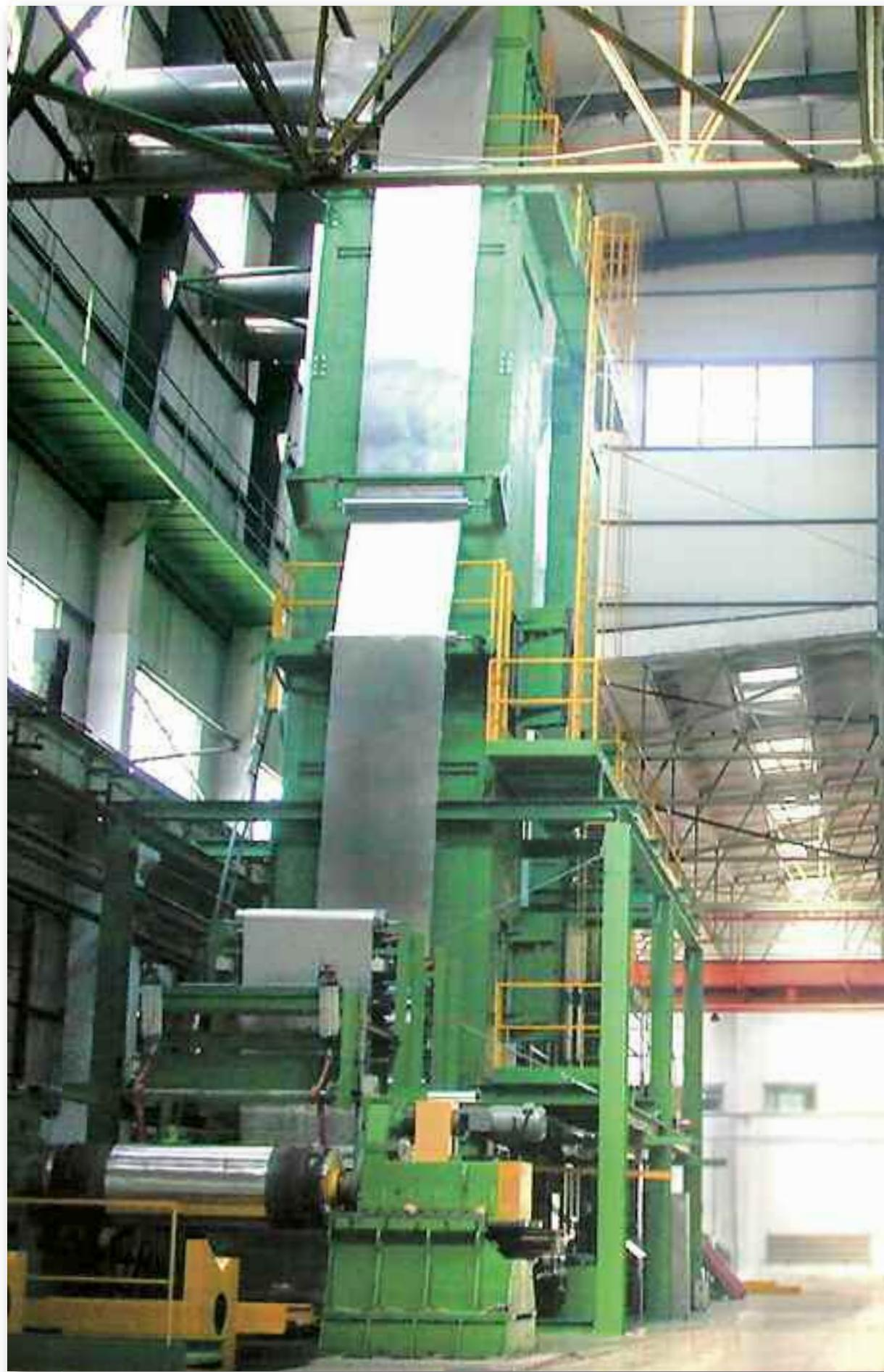
*Vertical plant for the treatment of the "fin stock" aluminium belt surface
