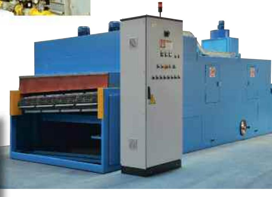
Washing machine for pipes
